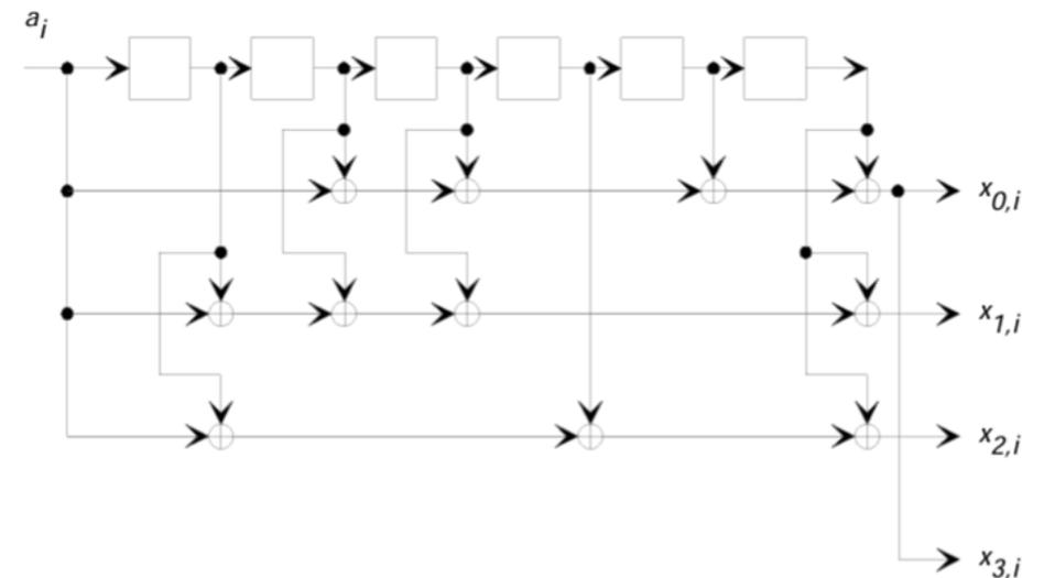
Figure 86: Convolutional encoder
